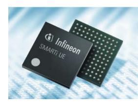
SMARTIUE IS THE FIRST single-chip dual-mode UMTS / EDGE Transceiver IC with 3G DigRF V3.09 standard interface for multi-media and feature-rich mobile devices. It integrates the functionality of a UMTS- and EDGE RF transceiver IC and the mixed signal blocks required for data conversion and RF control. With its standard pure digital interface to the baseband it makes the digital part independent from a specific RF implementation without the need for an additional analog baseband IC.
